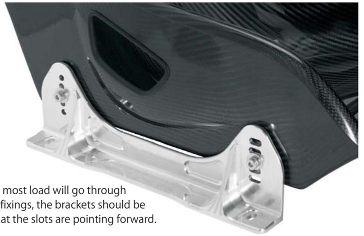
The TB FIA bracket system is designed to point outwards from the seat to give maximum stability. This also helps to place the seat on top of existing runner systems, although if used in racing we do not recommend using adjustment runners.
