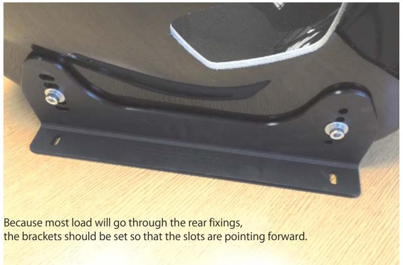
Because most load will go through the rear fixings, the brackets should be set so that the slots are pointing forward.
