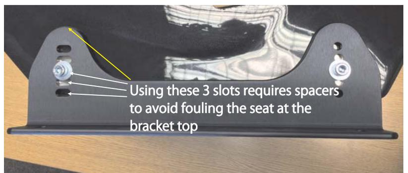
Using these 3 slots requires spacers to avoid fouling the seat at the bracket top
