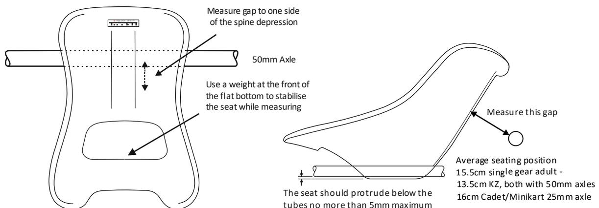
Be aware that Historic karts always had the seat set further away from the axle. Pre-2005 chassis with a 40mm diameter axle used around a 21.5cm gap and karts aged from 2005 to 2009 with a 50 mm axle approximately 18cm. If the kart has a 30 or 40mm axle you will need to compensate for this by changing the gap dimension accordingly.
