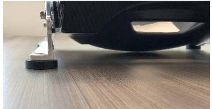
Set on the upper holes at the front middle hole at the rear with the base skimming the floor using 12 mm of spacers, the **A** dimension is 50.2 to 50.8 cm using only the slots to give adjustment.
