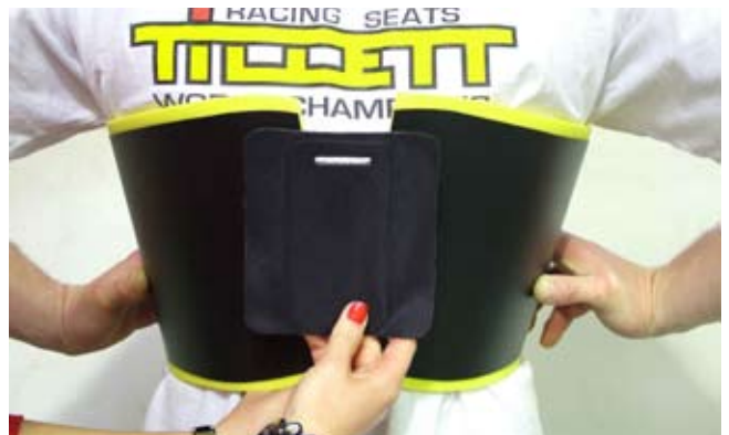
Get assistance in positioning the back joining panel. This will hold the two halves at the correct angle for your shape.
